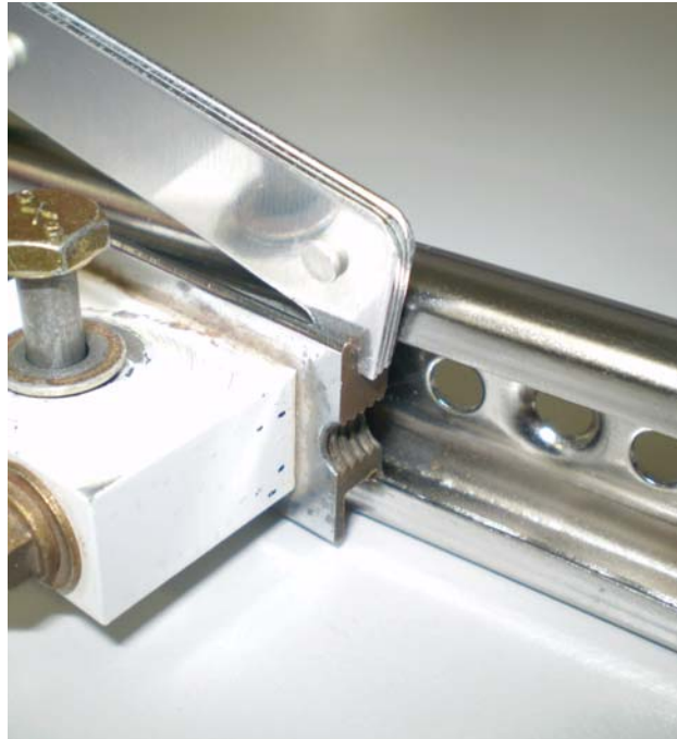
Figure 6: Forward Slide Gauge inserted between the slide and track, indicating a worn part. (Removed from aircraft for clarity only, checking can be done while installed)
