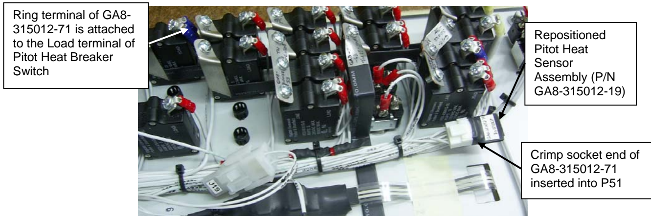
Figure 1. Correct installation of the relocated pitot heat sensor assembly and wiring
