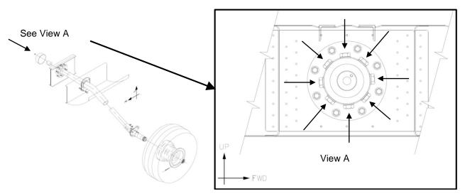
Figure 2 – Main Gear Leg Inboard Attachment Bolts
