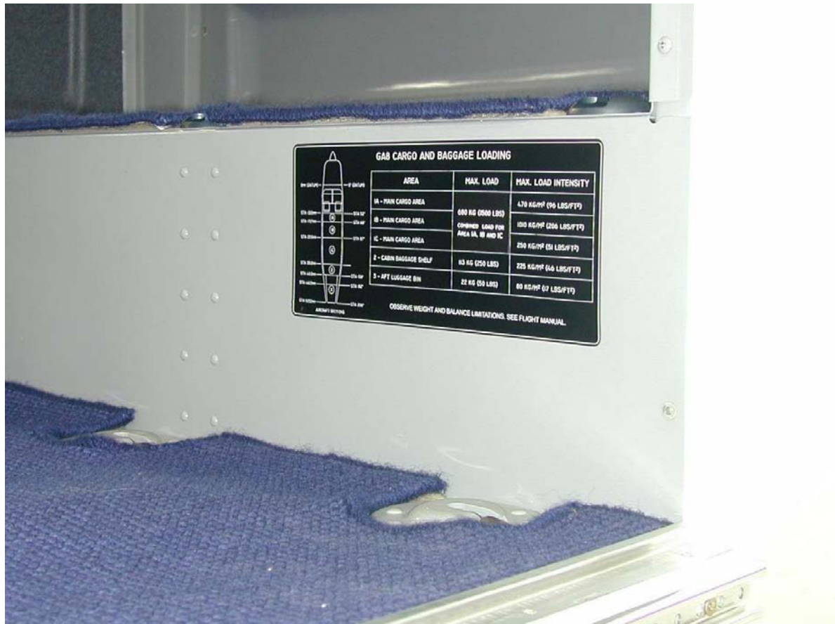
Figure 4-1 – Load placard location
