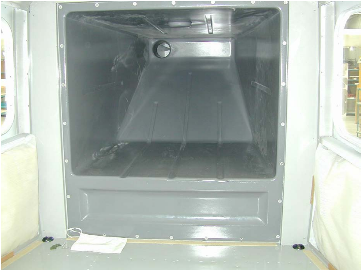
Figure 2-1 – Aft luggage bin installation
