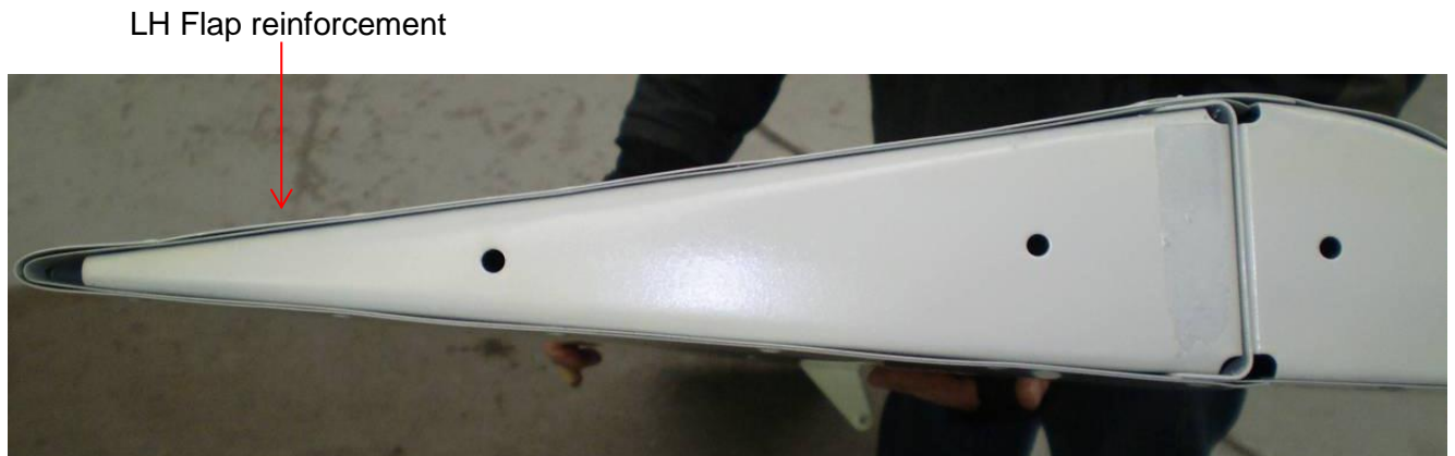
Figure 7 : LH flap skin reinforcement
