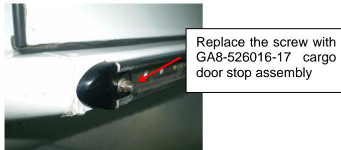
Figure 7: Fwd Door Stop Installation
