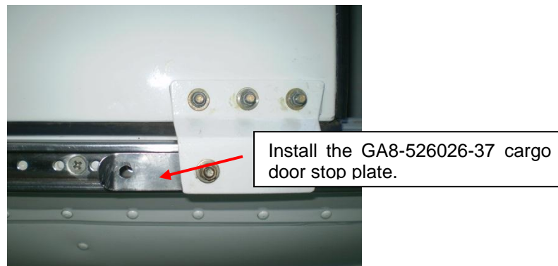
Figure 8: Fwd Door Stop Installation
