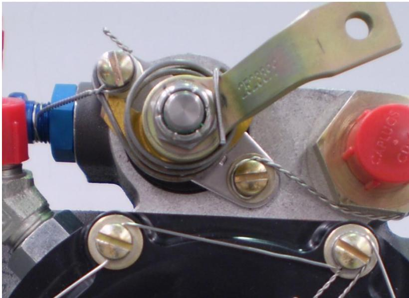
Figure 7: Installation of Mixture Side thicker spring
