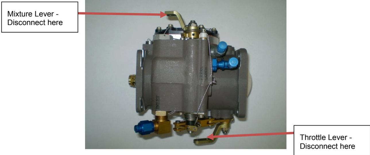
Figure 1: Throttle and Mixture control lever locations
