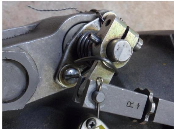
Figure 6: Installation of Throttle Side thicker spring
