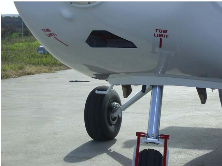
**Figure 2. An example of "Tow Limit" markings.**
